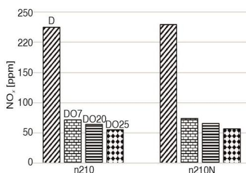
Figure 6. Exhaust emission of NO<sub>x</sub> for different fuels and engine loads, [ppm]
