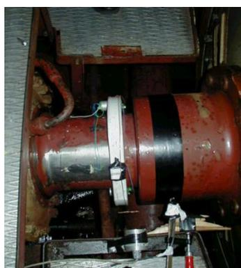
**Figure 1. Strain gauges mounted on the propeller shaft**
