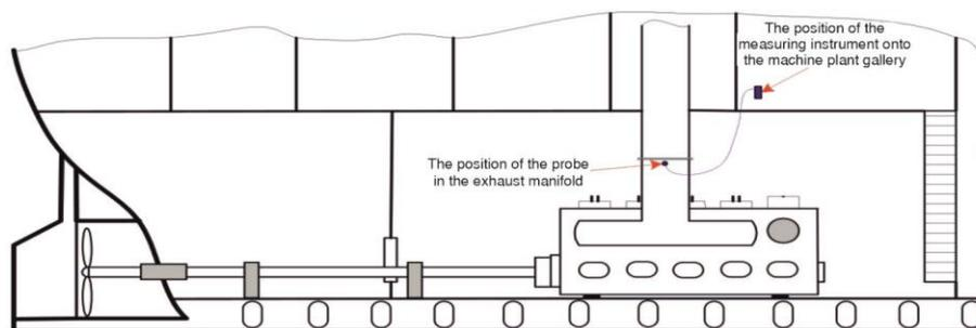
Figure 2. The position of exhaust emission testing equipment
