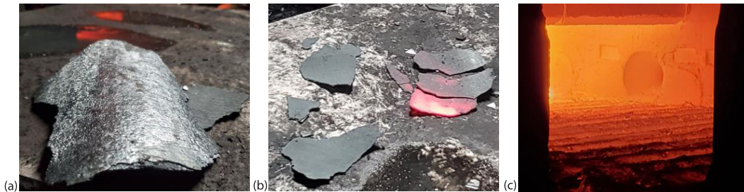
Figure 16. Iron oxide scales dropped from billets and hearth photo taken through charging door
