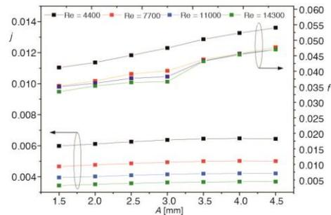
**Figure 6. Impact of wave amplitude on Colburn and friction factors**
