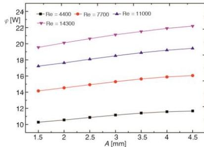
**Figure 5. Wave amplitude's effect on thermal flux**
