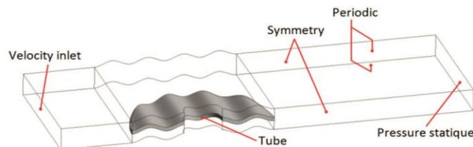
Figure 2. The 3-D Computational domain with its prescribed boundary conditions
