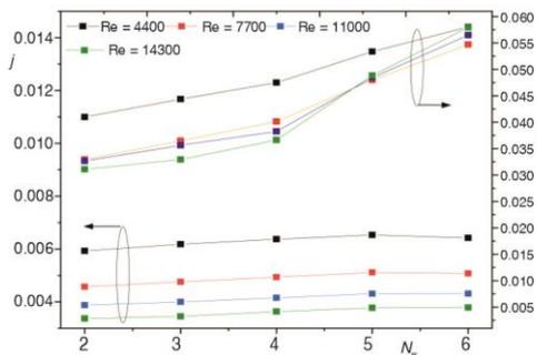
**Figure 9. Impact of wave number on Colburn and friction factors**
