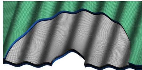
Figure 3. Generated mesh in the present simulations
