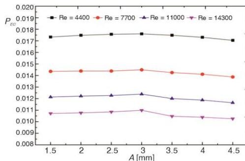
**Figure 7. Wave amplitude's effect on performance evaluation criteria**
