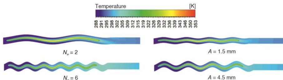
Figure 4. Temperature contours in wavy annular fin for two situations
