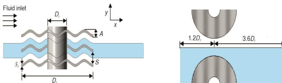
Figure 1. The researched wavy annular finned-tube HE geometric properties
