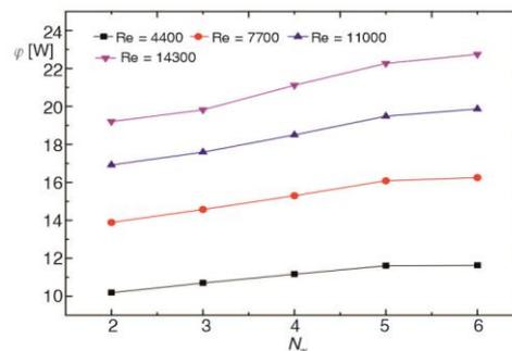
**Figure 8. Wave number's effect on thermal flux**
