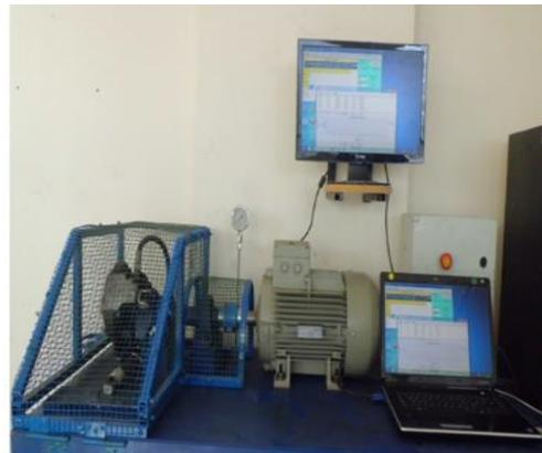
Figure 1. Image of brake pad friction wear tester
