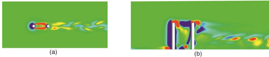
Figure 12. Instantaneous contours of the streamwise vorticity on a spanwise plane ( z/h = 0.5 ); (a) and a transverse plane ( y/W = 0.5 ) and (b) at S = 4.5
