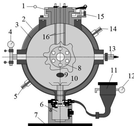
**Figure 1. Structure diagram of explosion pressure test equipment;** 1-sealing cap, 2-outer side of mezzanine, 3-inside of mezzanine, 4-vacuum gauge, 5-outlet of water, 6-mechanical two-way valve, 7-base, 8-observation window, 9-vacuum hole, 10-dispersion valve, 11-storage tank, 12-pressure gauge, 13-pressure sensor, 14-inlet of water, 15-limit switch, 16-ignition rod
