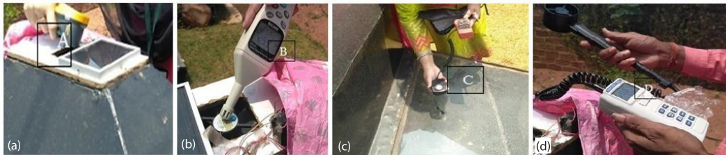
Figure 2. Measuring instruments; (a) infrared radiation pyrometer, (b) hygrometer, (c) light meter, and (d) anemometer
