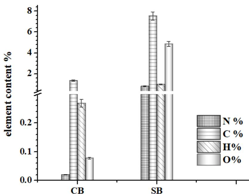
**Figure 4. The content of nitrogen, carbon, hydrogen and oxygen in fly ash samples from the cyclone (CB) and stack (SB)**
