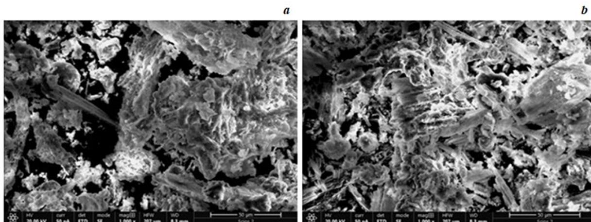
Figure 5. Scanning electron micrographs of fly ash from cyclone - CB (a) and stack - SB (b)
