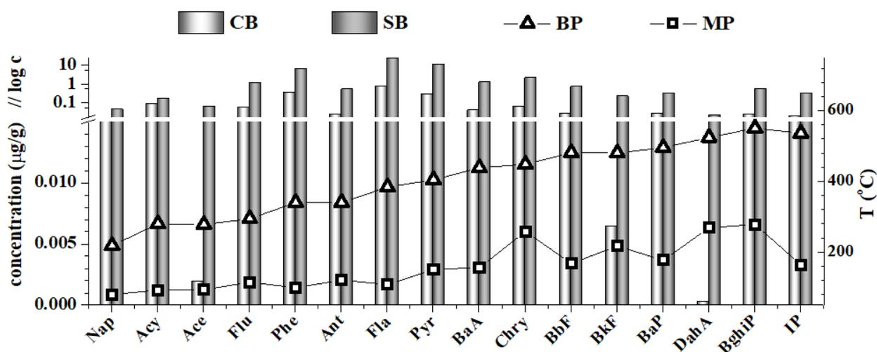
**Figure 6. PAH concentrations in biomass fly ash from the cyclone (CB) and stack (SB) parallel shown with their boiling points (BP) and melting points (MP)**
