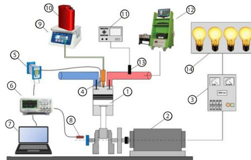
**Figure 3. Schematic of the experimental set-up;**
