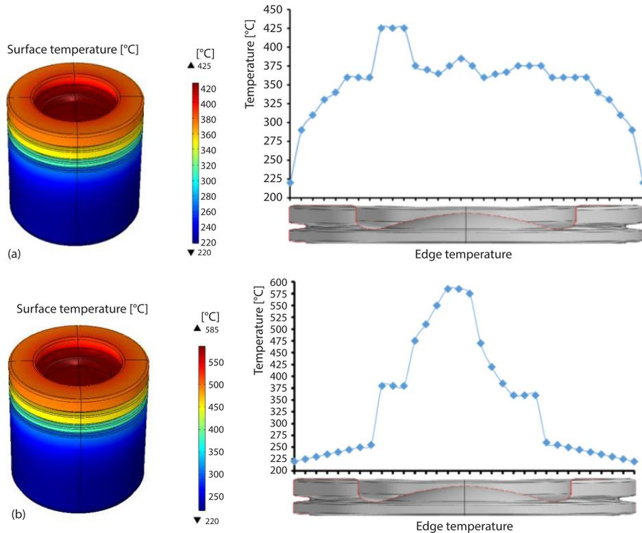
Figure 4. The results of the analysis of uncoated (a) and coated (b) pistons of the COMSOL program
