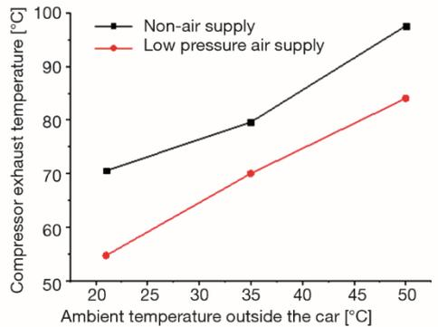
**Figure 4.** The compressor discharge temperature changes with the ambient temperature outside the car
