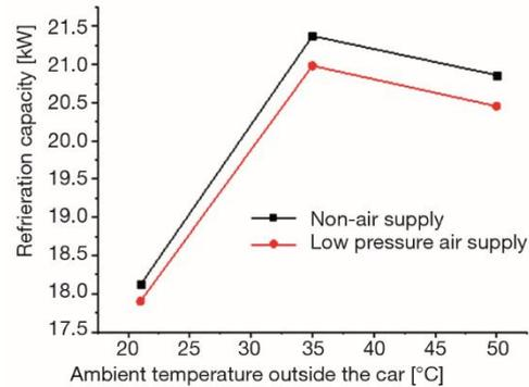
**Figure 5.** The cooling capacity of the system changes with the ambient temperature outside the car
