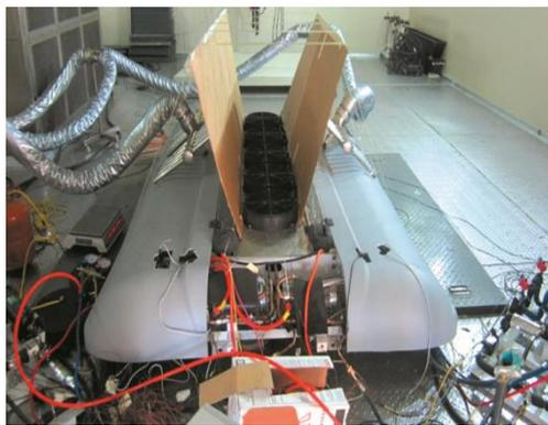
**Figure 3. The heat pump air conditioning system of a pure electric passenger car with low pressure supplemental air under test**
