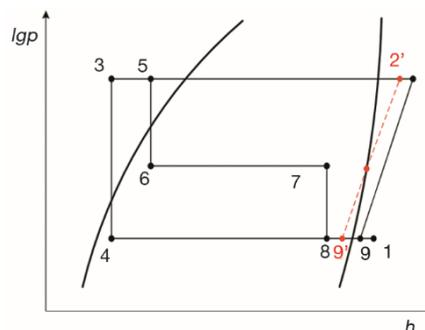
Figure 2. Low pressure supplemental gas theoretical cycle pressure enthalpy diagram
