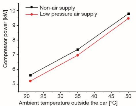
**Figure 6.** The change of system compressor power with the ambient temperature outside the car
