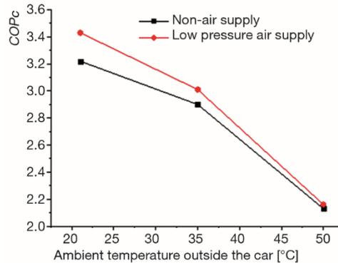
**Figure 7.** The change of system COPc with the ambient temperature outside the car
