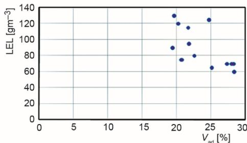
Figure 2. Evolutions of LEL with  $V_{ad}$  for fourteen kinds of coal dusts
