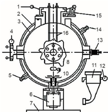
**Figure 1. The 20 L spherical vessels for explosion test;** 1 – sealed cap, 2 – outer jacket, 3 – inner jacket, 4 – vacuum meter, 5 – circulation water inlet, 6 – mechanical two-way valve, 7 – pedestal, 8 – sightglass, 9 – vacuum orifice, 10 – scattered valve, 11 – dust container, 12 – electro connecting pressure gauge, 13 – pressure sensor, 14 – circulation water outlet, 15 – safety and limit switches, 16 – ignition rod
