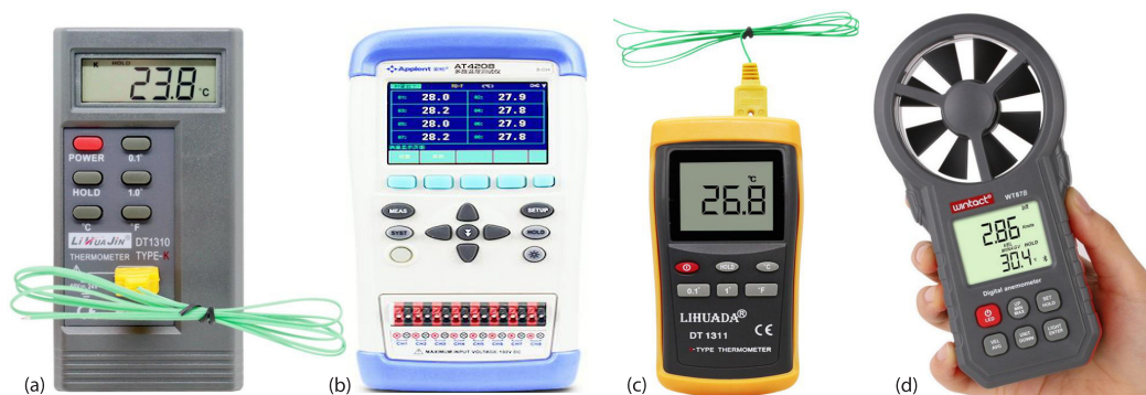
Figure 2. Physical diagram of the instrument; (a) Pde-ki long term data recorder (b) Pde-r4 four channel temperature data recorders, (c) temperature and heat flux measuring instrument, and (d) portable anemometer
