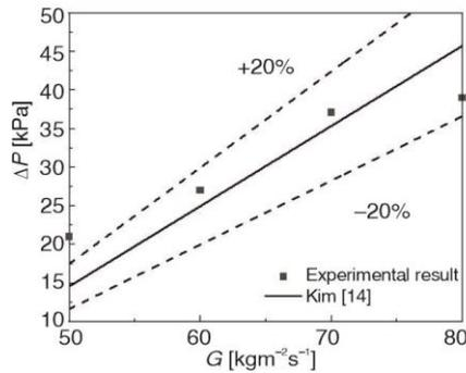
**Figure 4. Comparison of experimental result with Kim correlation for rectangular channel**
