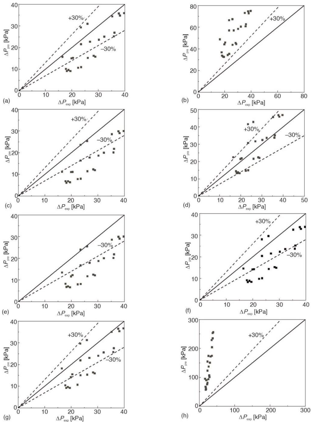
**Figure 6.** Comparison of experimental results with some related correlations; (a) L-M [17], (b) Chisholm [20], (c) Mishima and Hibiki [18], (d) Kim [14], (e) Lopez-Belchi [19], (f) Hossain *et al.* [21], (g) Sun and Mishima [22], and (h) Wilson *et al.* [23]
