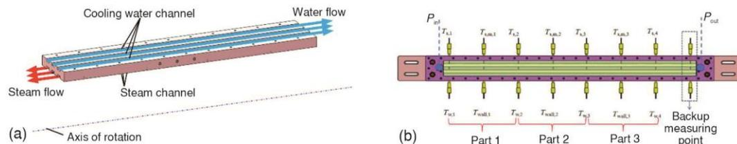
**Figure 3. Test section of experimental apparatus; (a) details of test section and (b) measurement point distribution in test section**
