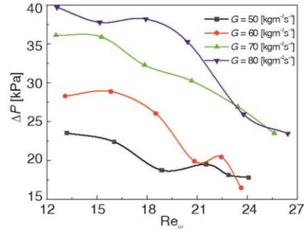
**Figure 5. Effect of  $Re_\omega$  on friction pressure drop**
