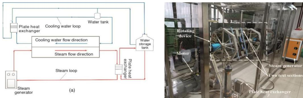
**Figure 2. Experimental apparatus; (a) schematic diagram of experimental apparatus and (b) site photo of experimental apparatus**
