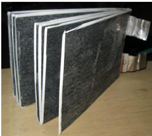
Figure 1. A disassembled prismatic pouch LIB cell
