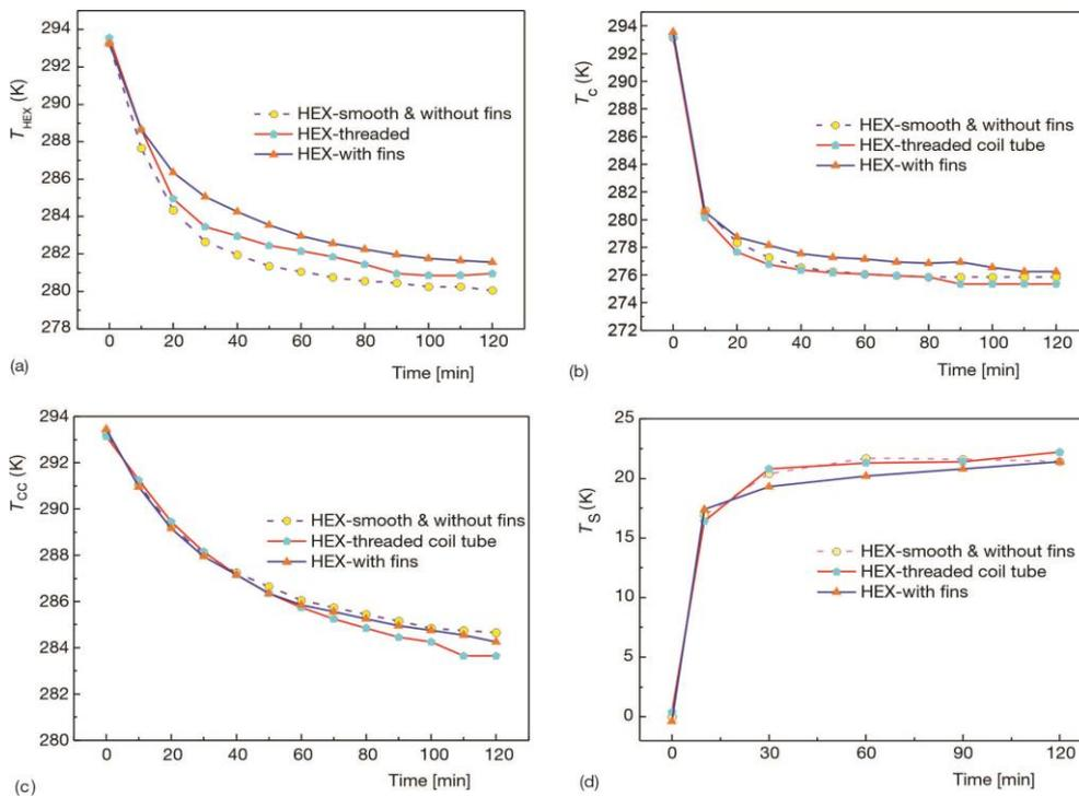
**Figure 10. Effect of inner and outer surface structures of heat exchange**
