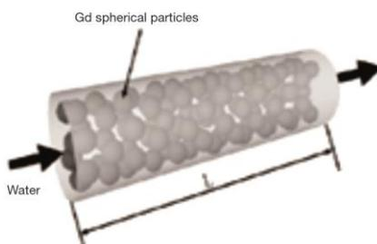
Figure 4. Schematic diagram of AMR filling
