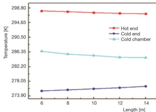
Figure 9. Temperature distribution vs. the tube length
