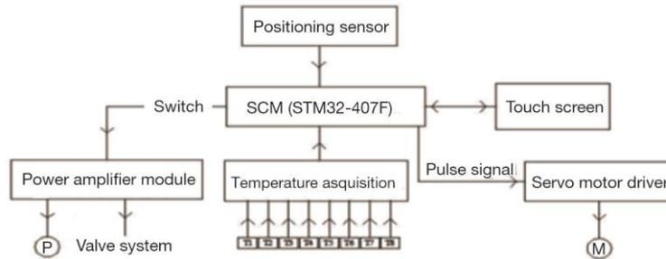
Figure 8. Magnetic refrigerator control structure diagram
