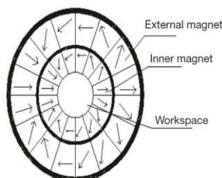
Figure 2. Structure diagram of double layer nested permanent magnet group
