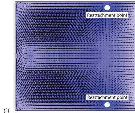
**Figure 5. Detailed Nusselt number ratio distributions for  $\phi = 0$  configuration at  $Re = 15500$  in a two-pass ribbed channel; (a) flat tape, (b)  $A/e = 0.5$ , (c)  $A/e = 1.0$ , (d)  $A/e = 1.5$ , (e)  $A/e = 2.0$ , and (f) velocity vectors along bottom surface for  $A/e = 1.5$**
