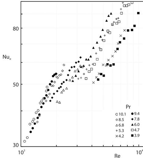
Figure 6. The variation of  $Nu_a$  with  $Re$  for different  $Pr$  ( $p/e = 6.7$ )
