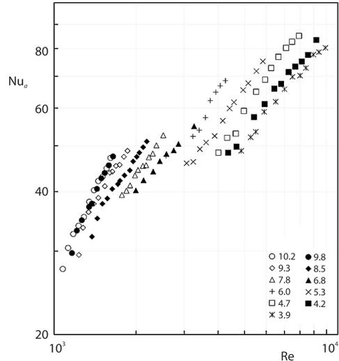
Figure 7. The variation of  $Nu_a$  with  $Re$  for different  $Pr$  ( $p/e = 15.0$ )
