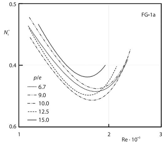
Figure 15. The variation of  $N_s^+$  ( $Q_* = Q_{*real}$ ) with  $Re$  for different  $p/e$ , ( $6.8 < Pr < 10.0$ )
