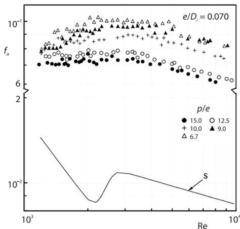
**Figure 1. The variation of friction factor with Re**
