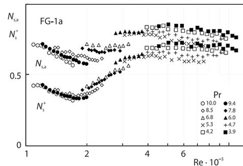
Figure 14. The variation of  $N_{s,a}$  and  $N_s^+$  with  $Re$  and  $Pr$  for  $Q_*^{real}$ ,  $p/e = 10.0$
