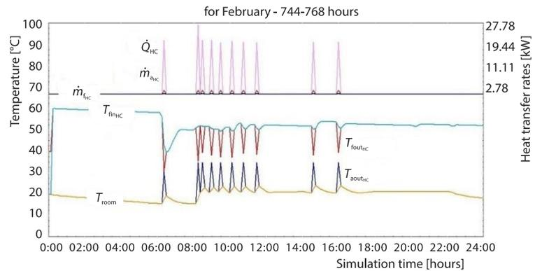
Figure 8. Changes of temperatures and heat transfer rates in the heating coil
