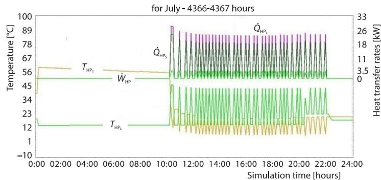
Figure 9. Changes of temperature and heat transfer rates of the heat pump
