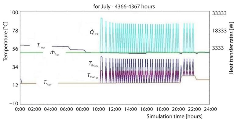
Figure 14. Changes of temperature and heat transfer rates of HEX
