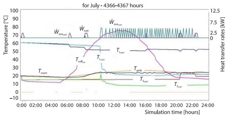
Figure 10. Temperature changes in HWT and CWT
