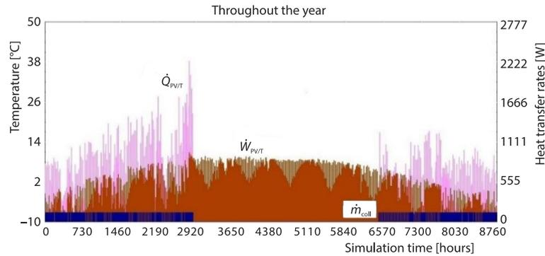
Figure 12. Changes of temperature, energy, and power of the PV/T collector throughout the year
