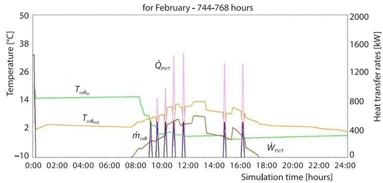
Figure 7. Changes in temperature, energy, and power of the PV/T collector
