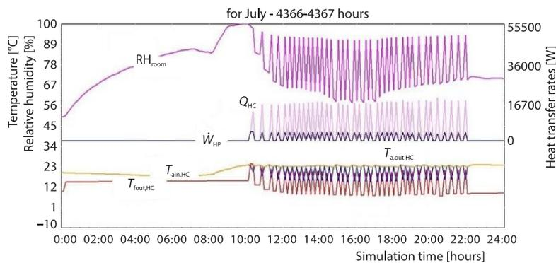
Figure 13. Changes in temperature and amount of heat transfer in the cooling coil
