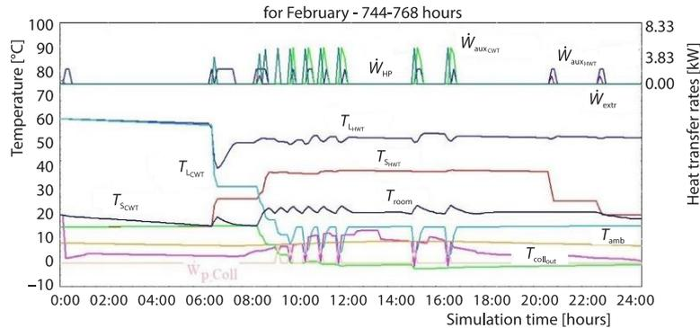
**Figure 6. Temperature changes in HWT and CWT**
