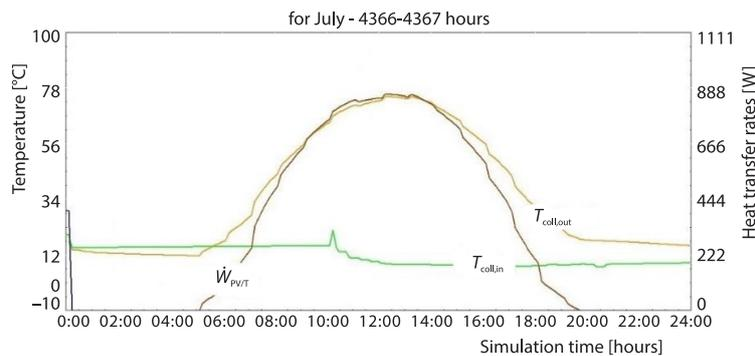
Figure 11. Changes of temperature, energy, and power of the PV/T collector
