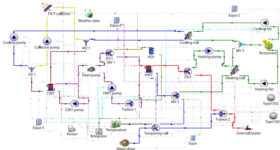
Figure 3. The TRNSYS model of the system
