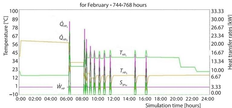
Figure 5. Changes of temperature and heat transfer rates of the heat pump
