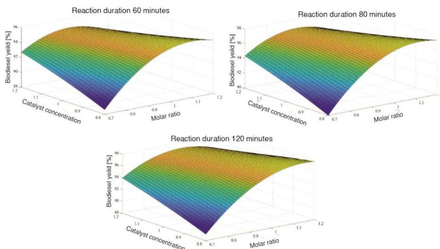
Figure 7. Influence of catalyst loading and molar ratio at various reaction duration
