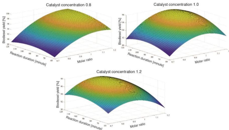
Figure 5. Influence of molar ratio and reaction duration at various catalyst loading
