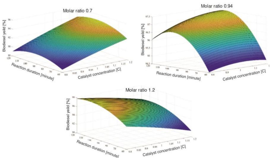
Figure 6. Influence of reaction duration and catalyst loading at various molar ratio
