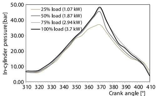
**Figure 11. In-cylinder pressure profile during compression and combustion phase for D + CNG + HHO operation**
