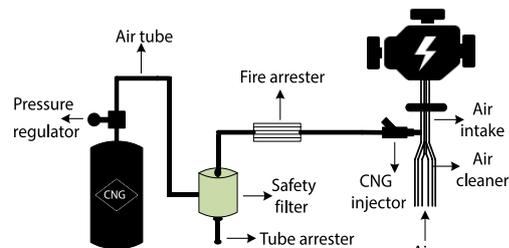
**Figure 3. The CNG injection circuit**
