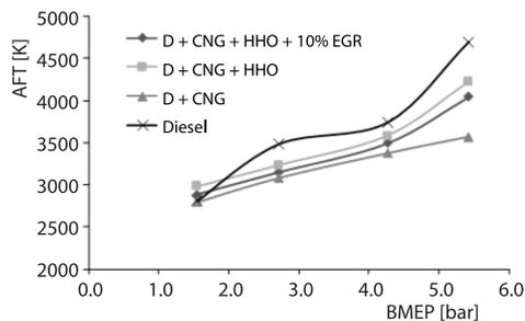
**Figure 9. Adiabatic temperature of the fuel mixture combination with BMEP**
