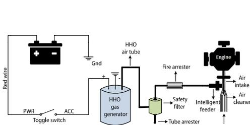
**Figure 2. Browns gas (HHO) generation lay-out**
