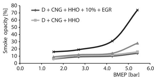
Figure 17. Smoke opacity with BMEP
