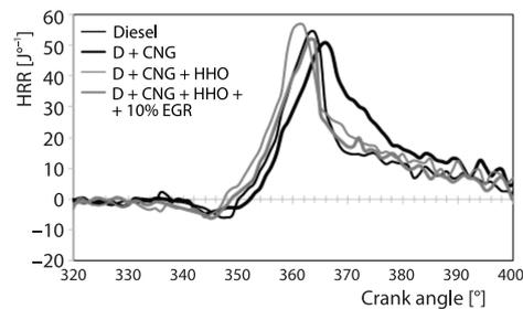
**Figure 8. Heat release rate vs. crank angle for various fuels combinations at full load**
