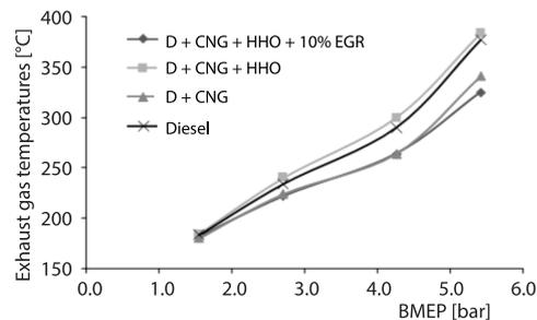
**Figure 10. Exhaust gas temperature of the fuel mixture combination with BMEP**
