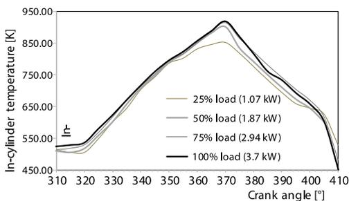
**Figure 13. Temperature profile during compression and combustion phase for D + CNG + HHO operation**
