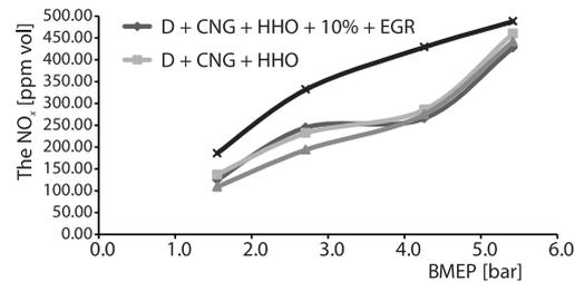
Figure 14. The  $\text{NO}_x$  with BMEP
