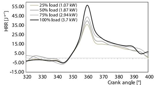
**Figure 12. The HRR profile during compression and combustion phase for D+CNG+HHO operation**
