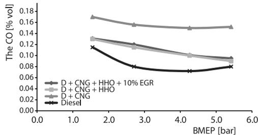
Figure 16. The CO emission with BMEP
