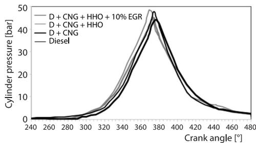
**Figure 7. In-cylinder pressure vs. crank angle for various fuels combinations at full load**
