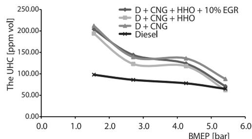
Figure 15. The UHC emission with BMEP
