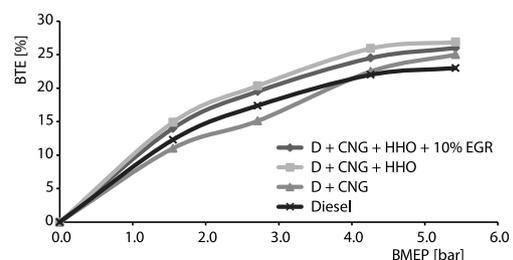
Figure 5. The BTE with BMEP
