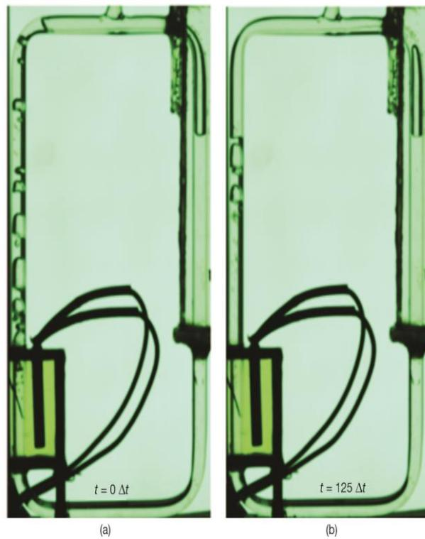
**Figure 10.** Flow process of a vibrational TPLT with filling ratio = 70%; (a)  $t = 0\Delta t$  and (b)  $t = 125\Delta t$
