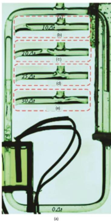
**Figure 5. Flow process of a static TPLT with filling ratio = 60%;**
