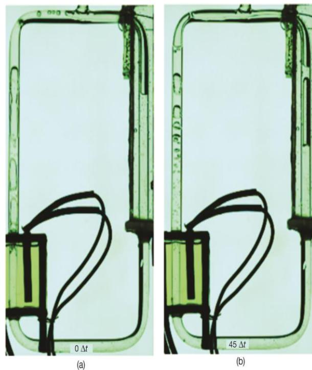
**Figure 6. Flow process of a static TPLT with filling ratio = 70%;**
