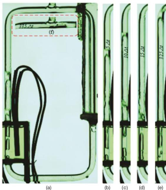
**Figure 3.** Flow process of a static TPLT with filling ratio = 40%; (a)  $t = 0\Delta t$ , (b)  $t = 5\Delta t$ , (c)  $t = 10\Delta t$ , (d)  $t = 15\Delta t$ , (e)  $t = 325\Delta t$ , and (f)  $t = 335\Delta t$
