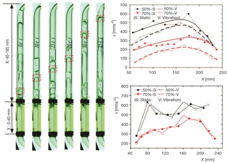
**Figure 11.** Velocity distribution of the TPLT; (a) definition of  $X$ , (b)  $P = 20\text{ W}$ , and (c)  $P = 40\text{ W}$
