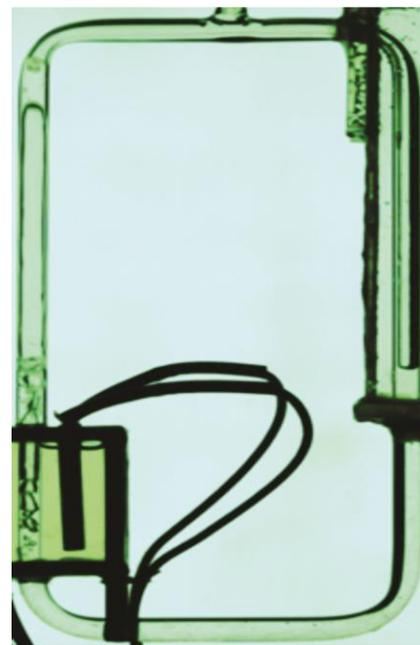
**Figure 4.** Flow process of a static TPLT with filling ratio = 50
