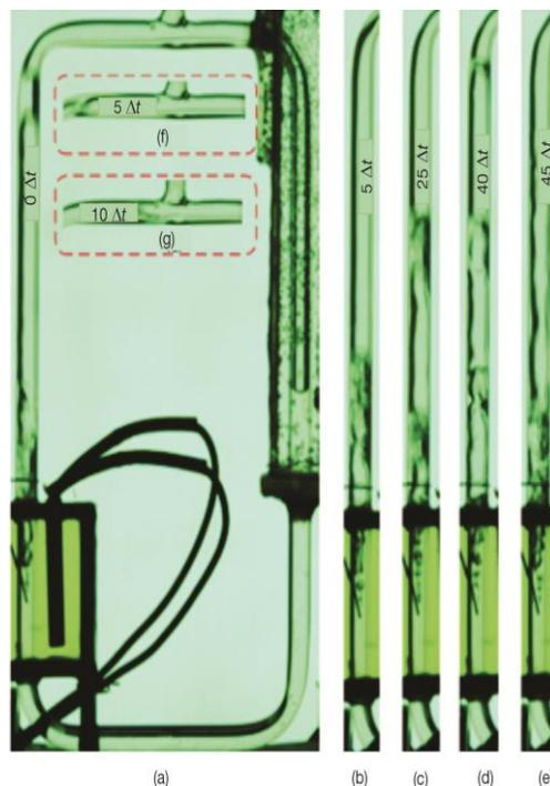
**Figure 8. Flow process of a vibrational TPLT with filling ratio = 50%; (a)  $t = 0\Delta t$ , (b)  $t = 5\Delta t$ , (c)  $t = 25\Delta t$ , (d)  $t = 40\Delta t$ , (e)  $t = 45\Delta t$ , (f)  $t = 5\Delta t$ , and (g)  $t = 10\Delta t$**
