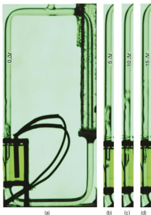
**Figure 7. Flow process of a vibrational TPLT with filling ratio = 40%; (a)  $t = 0\Delta t$ , (b)  $t = 5\Delta t$ , (c)  $t = 10\Delta t$ , and (d)  $t = 15\Delta t$**
