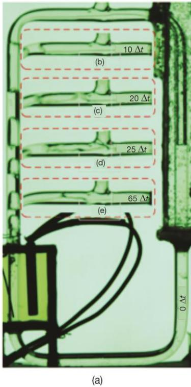
**Figure 9.** Flow process of a vibrational TPLT with filling ratio = 60%; (a)  $t = 0\Delta t$ , (b)  $t = 10\Delta t$ , (c)  $t = 20\Delta t$ , (d)  $t = 25\Delta t$ , and (e)  $t = 65\Delta t$
