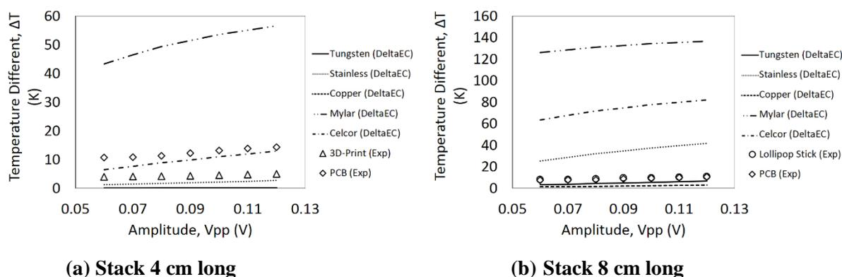
**Figure 5. The impact of stack's material temperature drop across stack length of (a) 4 cm (b) is 8cm long inside resonator of 0.385 m long**
