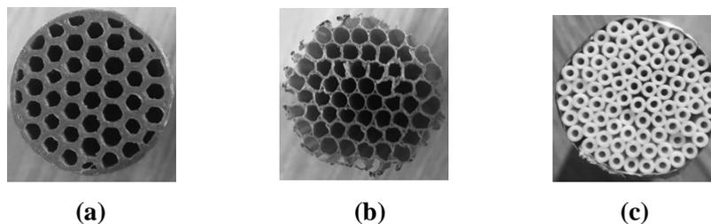
**Figure 3.** The porous structure is made of (a) Acrylonitrile Butadiene Styrene (ABS), (b) Polycarbonate foam (PCB), and (c) Lollipop stick
