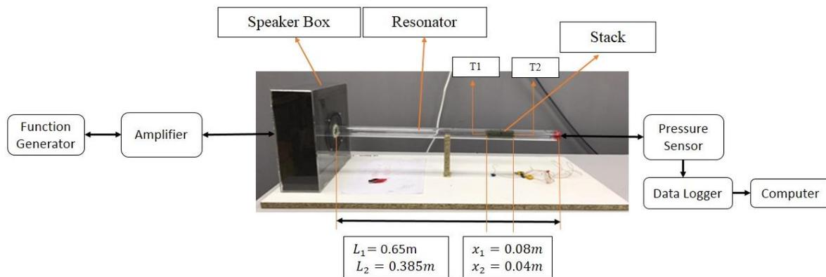
**Figure 2.** The experimental apparatus of the thermoacoustic cooler
