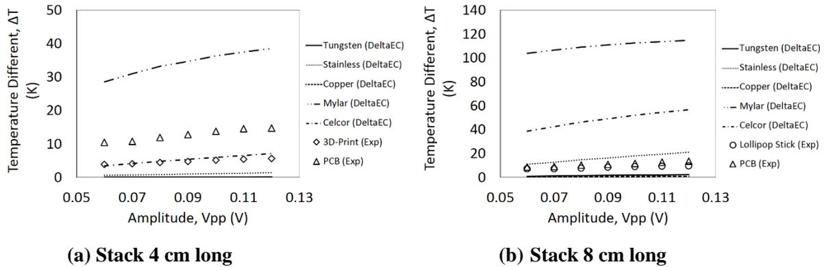
**Figure 4. The impact of stack's material on temperature drops across stack length of (a) 4 cm and (b) is 8 cm long inside resonator of 0.65 m long**
