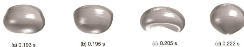
Figure 12. The profile of the bubble when crossing interface ( r = 2.5 mm)
