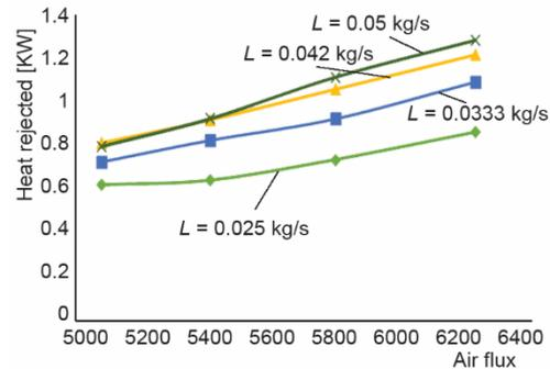
Figure 6. Heat rejected at the inlet water temperature of 40 °C
