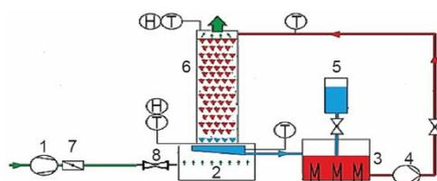
**Figure 3. Schematic of the experimental set-up:** 1 – air blower, 2 – air inlet-chamber, 3 – water heating tank, 4 – water pump, 5 – make-up tank, 6 – packed cooling tower, 7 – electronic controller unit, 8 – venturi meter, H – Humidity sensors, and T – temperature sensors
