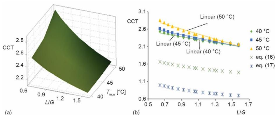
**Figure 4. The CCT vs. flow ratio at different temperature; (a) surface plot and (b) compared to other researches (for color image see journal web site)**
