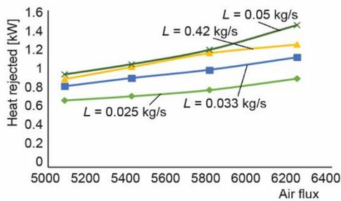
Figure 7. Heat rejected at the inlet water temperature of 45 °C
