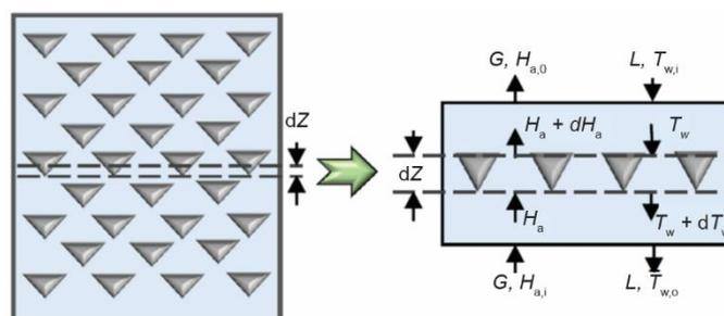
Figure 1. The process of transfer in the splash fills cooling tower
