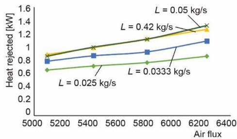
Figure 8. Heat rejected at the inlet water temperature of 50 °C
