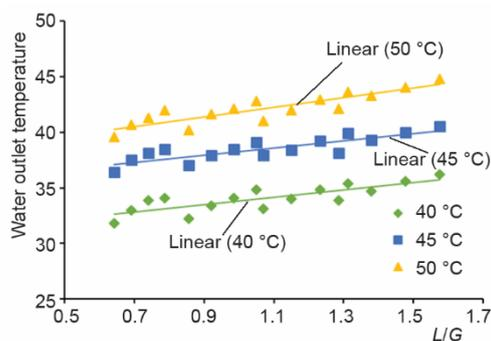
**Figure 5. Variation of outlet water temperature with the variation inlet water temperature and flow ratio**
