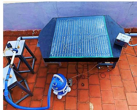
**Figure 2. Experimental set-up of SAH**
