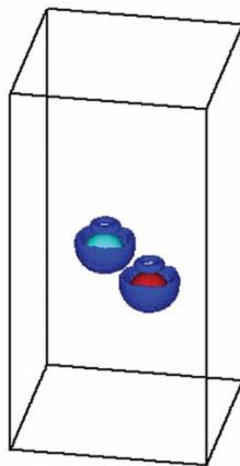
Figure 3. Reference results for  $\theta_0 = 5^\circ$  (Re = 120), the surface where  $\lambda_2 = -0.0004$
