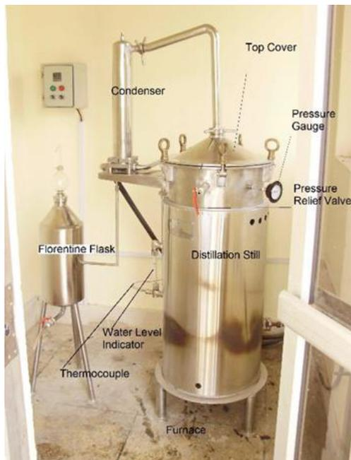
**Figure 3.** Pictorial representation of the controlled distillation system
