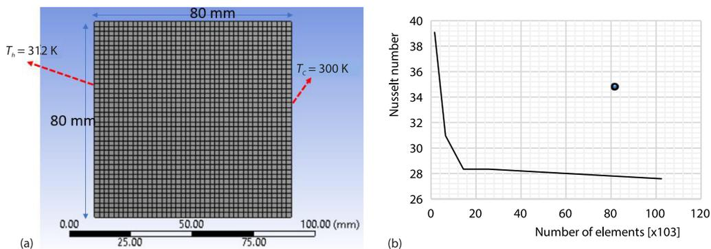
**Figure 3. (a) Mesh grid for sensitivity analysis and (b) variation of Nusselt number with mesh size**
