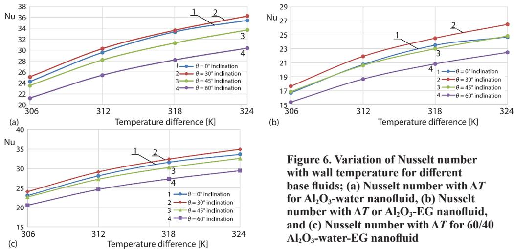
**Figure 6.** Variation of Nusselt number with wall temperature for different base fluids; (a) Nusselt number with  $\Delta T$  for  $\text{Al}_2\text{O}_3$ -water nanofluent, (b) Nusselt number with  $\Delta T$  or  $\text{Al}_2\text{O}_3$ -EG nanofluent, and (c) Nusselt number with  $\Delta T$  for 60/40  $\text{Al}_2\text{O}_3$ -water-EG nanofluent
