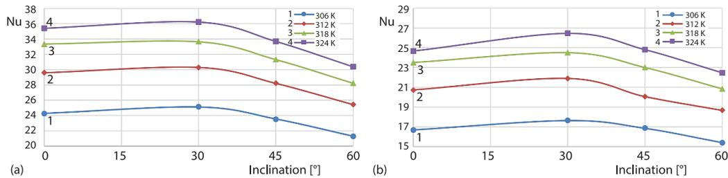
**Figure 7. Variation of Nusselt number for different wall temperature at different inclinations;**
