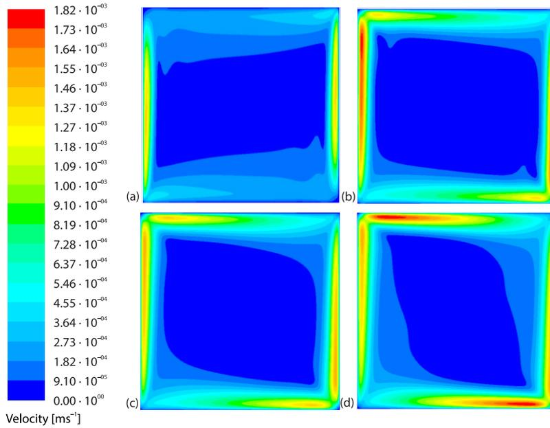
**Figure 5.** Velocity contour for  $\Phi = 3\%$   $\text{Al}_2\text{O}_3$ -water and 312 K hot wall temperature; (a)  $\theta = 0^\circ$  inclination, (b)  $\theta = 30^\circ$  inclination, (c)  $\theta = 45^\circ$  inclination, and (d)  $\theta = 60^\circ$  inclination
