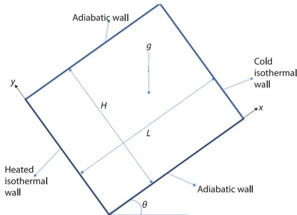
Figure 1. Model geometry with boundary conditions
