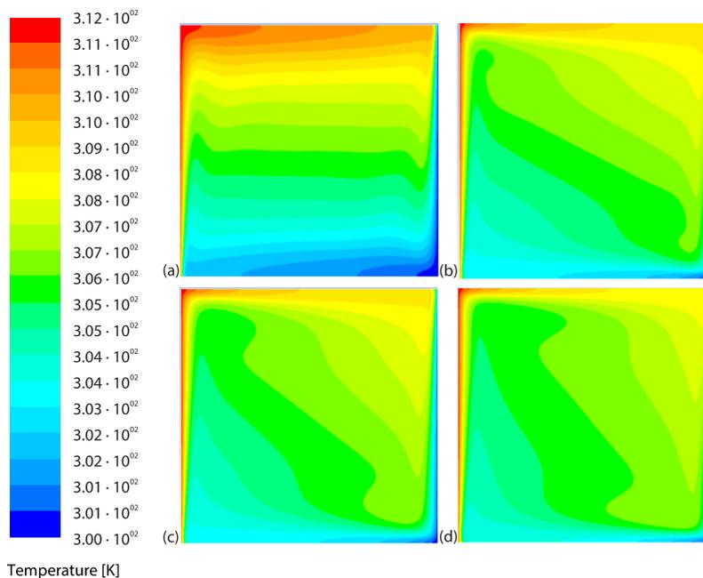
**Figure 4. Temperature contour for  $\Phi = 3\%$  Al<sub>2</sub>O<sub>3</sub>-water and 312 K hot wall temperature; (a)  $\theta = 0^\circ$  inclination, (b)  $\theta = 30^\circ$  inclination, (c)  $\theta = 45^\circ$  inclination, and (d)  $\theta = 60^\circ$  inclination**
