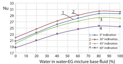
**Figure 8. Variation of Nusselt number with change in base fluid composition at different inclinations**
