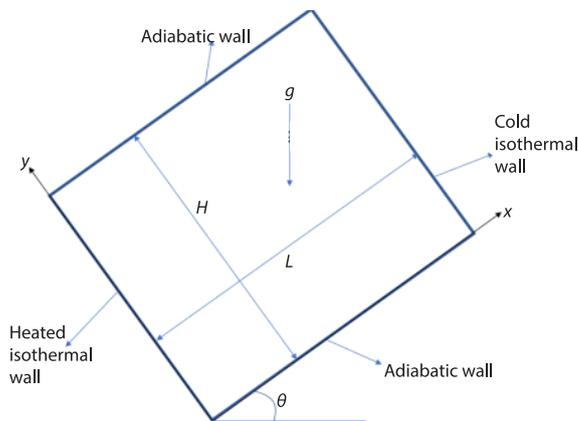
Figure 1. Model geometry with boundary conditions
