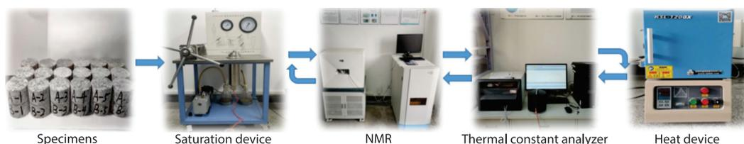
Figure 1. Test procedures and equipment
