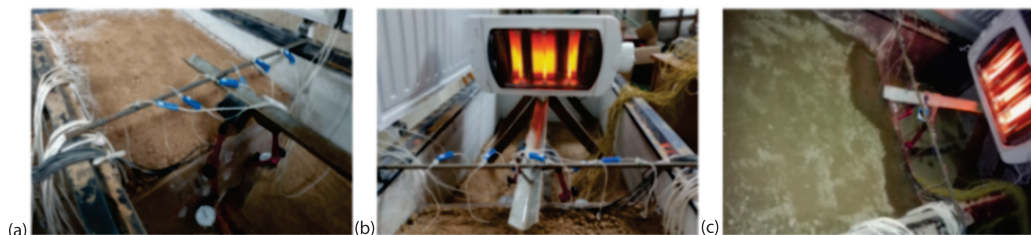
Figure 6. Model test process diagram; (a) freeze, (b) melt, and (c) water supply
