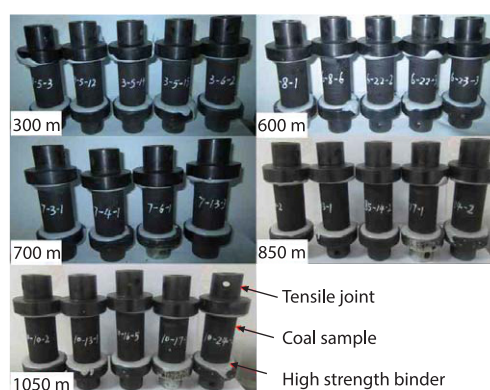
Figure 2. Bonded samples obtained at different mine depths
