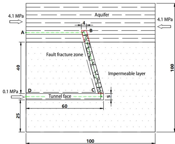
**Figure 1. Numerical model of water inrush in karst fault tunnel**
