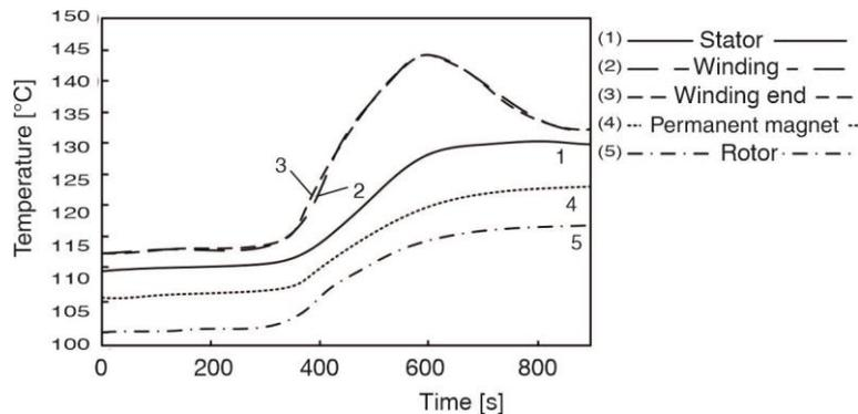
**Figure 2. Temperature change curve of various parts of motor under two times of overload current**
