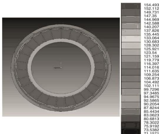
**Figure 1. Temperature distribution of 240 seconds operation with two times overload current and overload**
