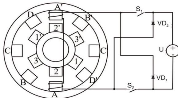
Figure 1. Four-phase 8/6-pole structure SRM structure
