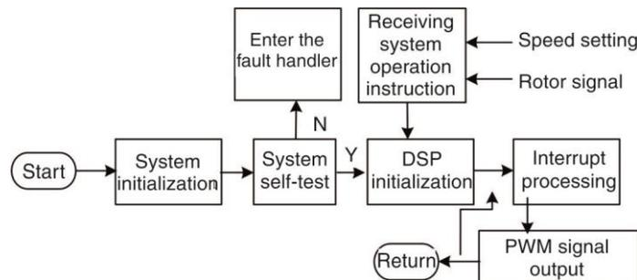
Figure 2. System operation main block diagram
