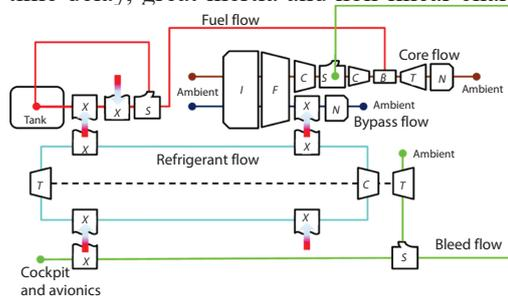
Figure 1. The PEMFC thermal management system model block diagram
