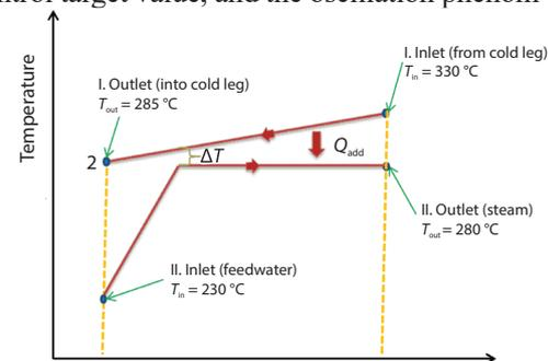
Figure 9. Temperature and temperature difference fluctuation degree of inlet and outlet cooling water of the electric reactor
