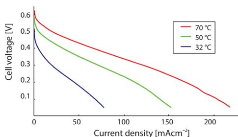
**Figure 1.** The DMFC voltage/current density curve at different temperatures
