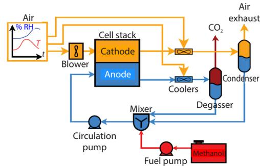
**Figure 2. The DMFC system identification block diagram**
