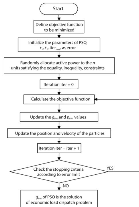
**Figure 1. Flow chart of the particle swarm optimization algorithm**
