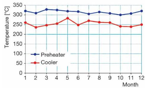
**Figure 6. Monthly variation of exhaust gas temperature from the preheater and cooler**
