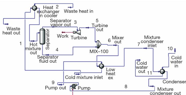
Figure 8. Kalina cycle integration and layout using ASPEN software
