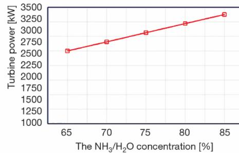
**Figure 11. Effect of NH<sub>3</sub>-H<sub>2</sub>O concentration on turbine power**
