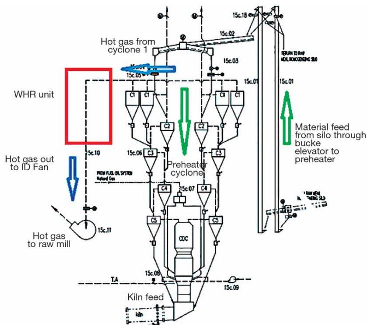
Figure 1. Flow diagram for preheater area and WHR system position, preheater
