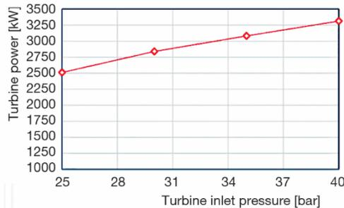
**Figure 10. Effect of turbine inlet pressure on turbine power**
