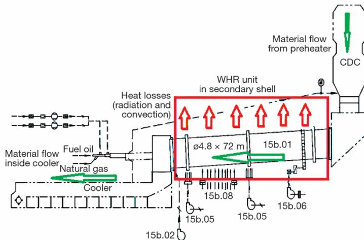
Figure 2. Flow diagram for kiln area and proposed WHR system position, kiln
