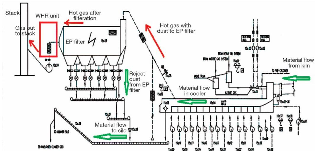
Figure 3. Flow diagram for the cooler area and proposed WHR system position, cooler
