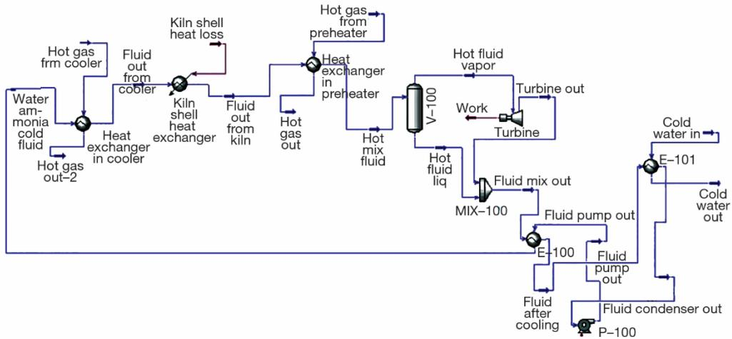
**Figure 13. Kalina cycle driven by combination of waste heat from cooler, preheater, and kiln**
