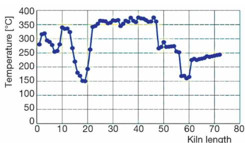
**Figure 5. Variation of average measured temperature along kiln shell during normal operation**
