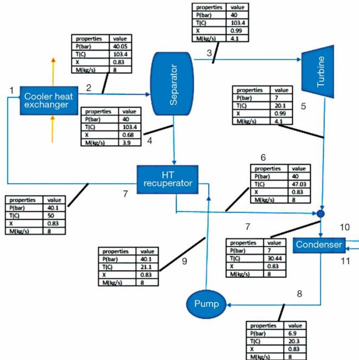
**Figure 12. The ASPEN simulation results for WHR from kiln using Kalina cycle**
