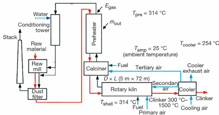
Figure 4. Schematic diagram showing major WHR sources from cement production lines
