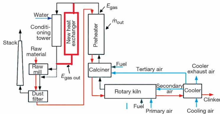
**Figure 7. Proposed location of heat exchanger for heat recovery from preheater exhaust gas**
