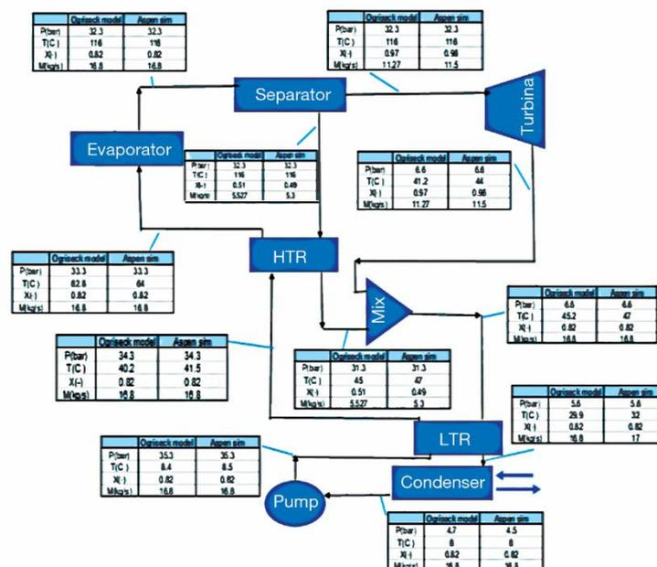
Figure 9. Kalina model validation, comparison with Sirko [14]
