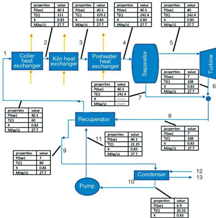
Figure 14. The ASPEN simulation results for combined WHR from cooler, preheater, and kiln using Kalina cycle
