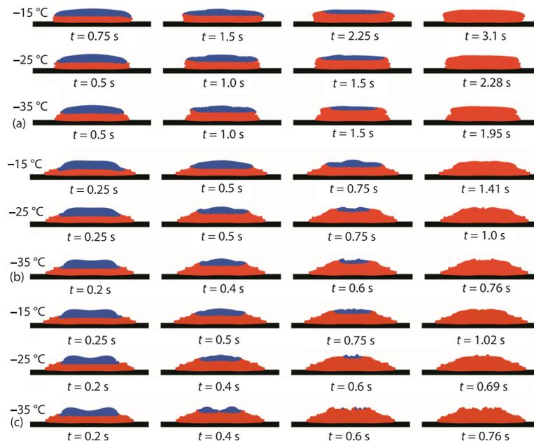
Figure 7. Cloud charts of droplet freezing under different temperatures; (a) 1.0 m/s cloud chart of frozen droplets, (b) 1.7 m/s cloud chart of frozen droplets, and (c) 2.0 m/s cloud chart of frozen droplets
