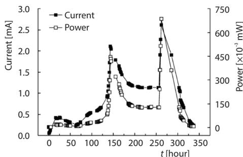
**Figure 6. Current and output power changes over time**
