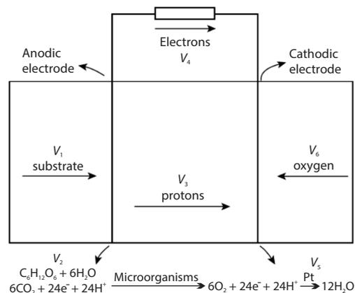
Figure 7. Schematic diagram of influencing factors of current
