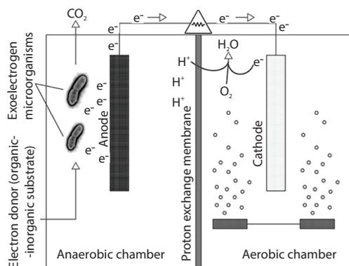
**Figure 1. Schematic diagram of the AMFC system**
