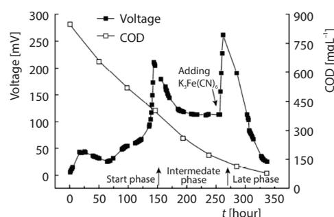
**Figure 4. Changes in output voltage and COD over time**
