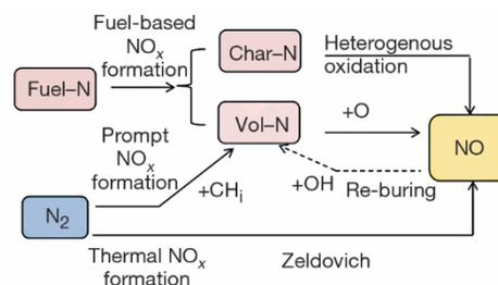
Figure 3. The  $\text{NO}_x$  formation mechanism in pulverized coal combustion
