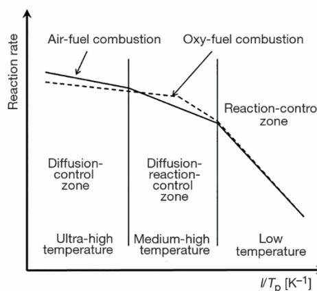
**Figure 2. Effect of temperature on the reaction rate of coal char**
