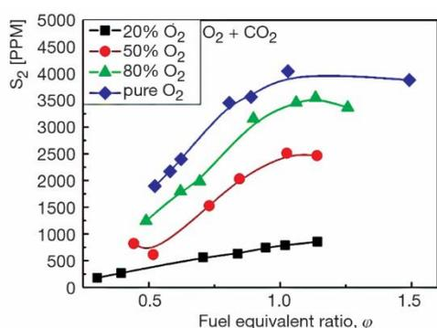
**Figure 4.** The influence of oxygen concentration and fuel equivalent ratio on SO<sub>2</sub> emission [26]
