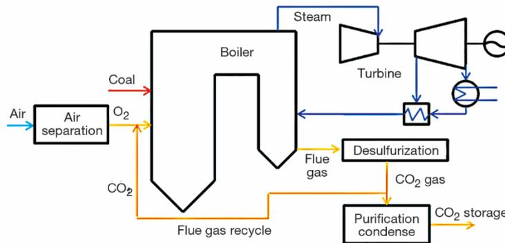
Figure 1. Schematic of oxy-coal combustion technology
