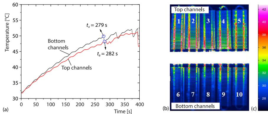
**Figure 4. The start-up performance when the inclination angle is  $0^\circ$ ; (a) temperature profile, (b) IR temperature profiles for start-up performance evaluation, and (c) the temperature scale is on the right**
