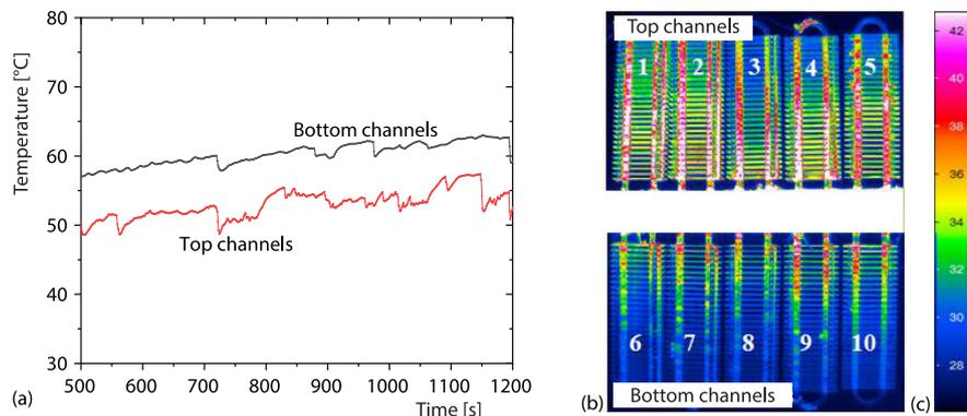
**Figure 7. The operation performance when the inclination angle is 0°; (a) temperature profile, (b) IR temperature profiles for operation performance evaluation, and (c) the temperature scale is on the right**
