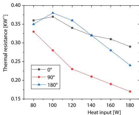
**Figure 10. Thermal resistance at inclination different angles**
