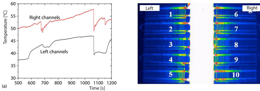
**Figure 9. The operation performance when the inclination angle is 180°; (a) temperature profile and (b) IR temperature profiles for operation performance evaluation**
