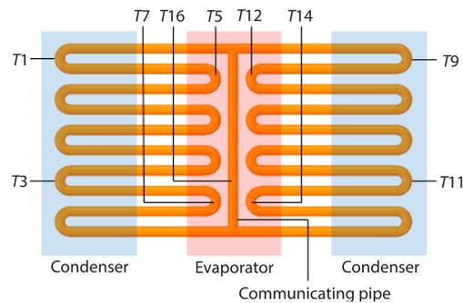
Figure 2. Temperature measuring points
