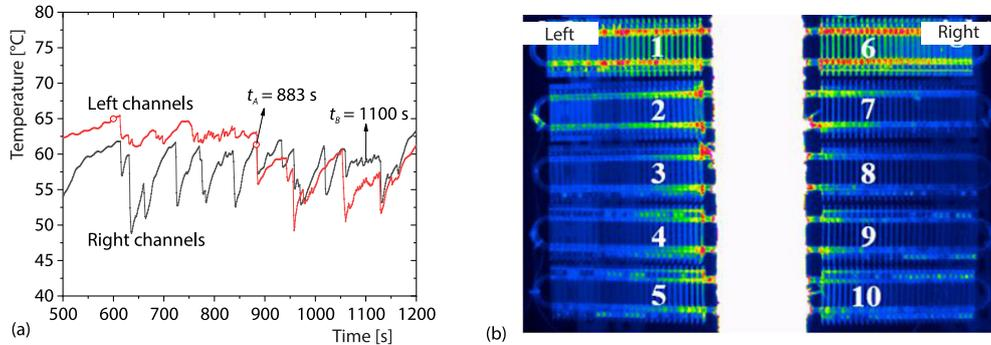
**Figure 8. The operation performance when the inclination angle is 90°; (a) temperature profile and (b) IR temperature profiles for operation performance evaluation**
