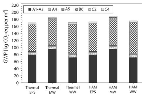
**Figure 4. The GWP of the materials of  $1 m^2$  wall construction with 15 cm ETICS**
