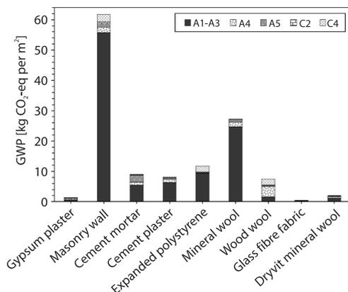
Figure 2. Embodied GWP of the materials of 1 m<sup>2</sup> wall construction with 15 cm ETICS
