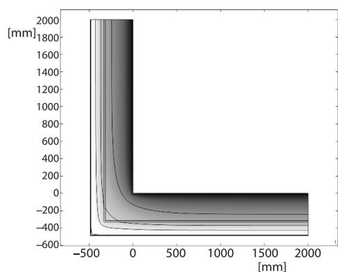
**Figure 6. Temperature distribution in wall corner with 15 cm WW based ETICS**
