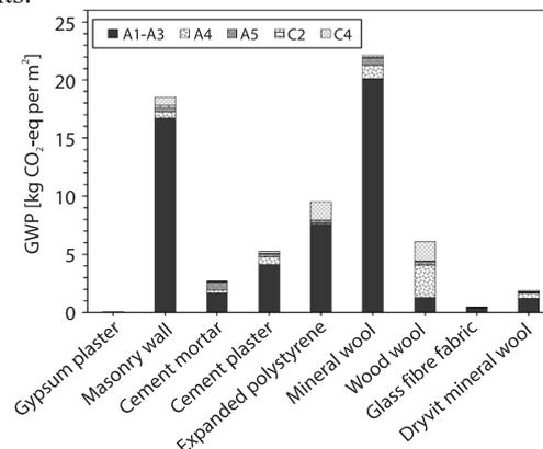
**Figure 3. Additional embodied GWP of the materials of 1 linear meter wall construction joint with 15 cm ETICS**
