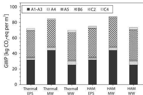
**Figure 5. Additional GWP of the materials of 1 meter wall construction joint, 15 cm ETICS**
