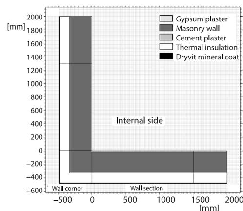
Figure 1. The 2-D model of an nZEB wall corner joint with 15 cm external thermal insulation system
