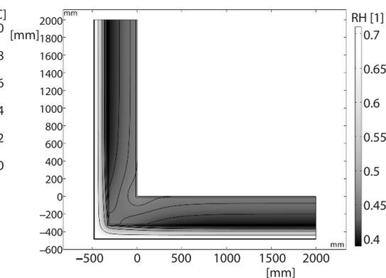
**Figure 7. Relative humidity distribution in wall corner with 15 cm WW based ETICS**
