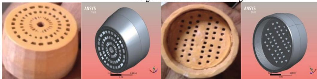
Figure 3. Front and backside view of the existing model and the newly fabricated nozzle aerator
