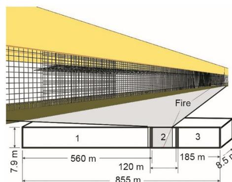
**Figure 1. Geometry and mesh set-up**
