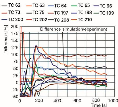
**Figure 3. Deviation of simulation results from experimental data [%] for 50 MW fire**
