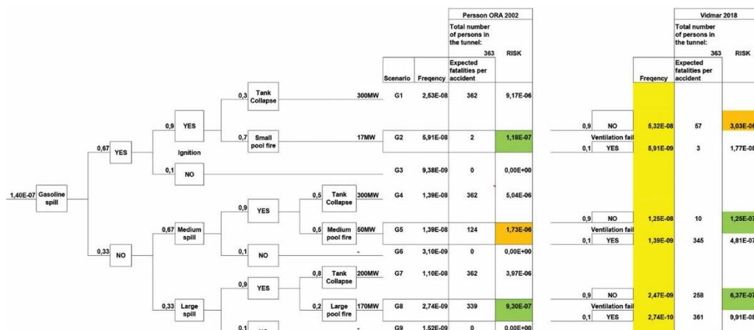
Figure 5. Event tree for gasoline spill
