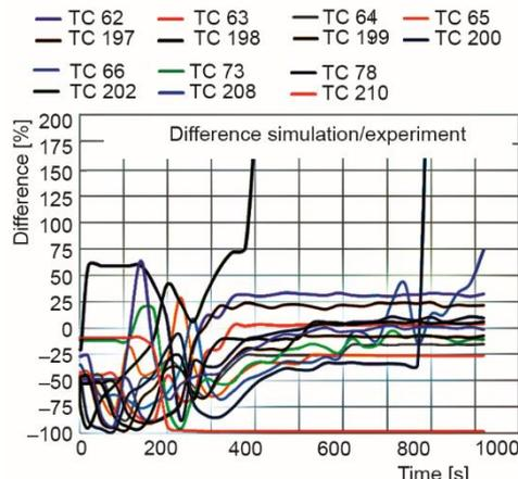
**Figure 4. Deviation of simulation results from experimental data [%] for 100 MW fire**
