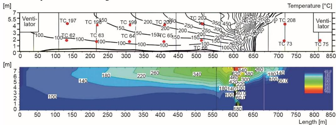
**Figure 2. Temperature field along the center of the tunnel for a 50 MW fire 15 minutes after ignition; experiment and simulation**
