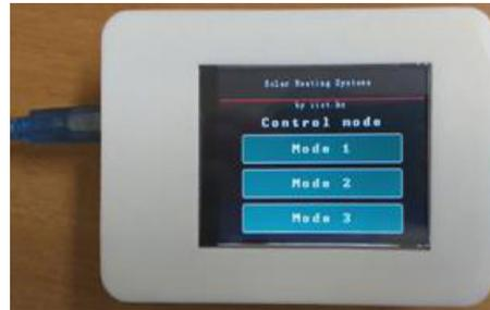
Figure 7. Solar system controller display
