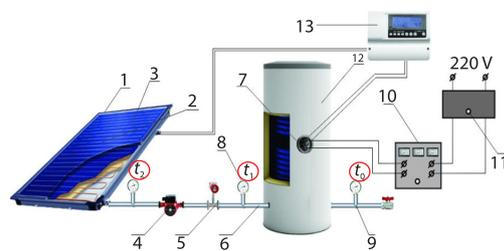
**Figure 2. Experimental installation of solar heat supply with master controller:** 1 – heat-insulated body, 2 – translucent coating, 3 – absorber tank, 4 – circulating pump, 5 – flowmeter, 6 – pipe-line, 7 – tubular heating element, 8, 9 – thermometers for measuring water temperature at inlet and outlet from absorber tank and environment, 10 – set of electric meters K 501, 11 – autotransformers, 12 – accumulator tank, and 13 – master controller
