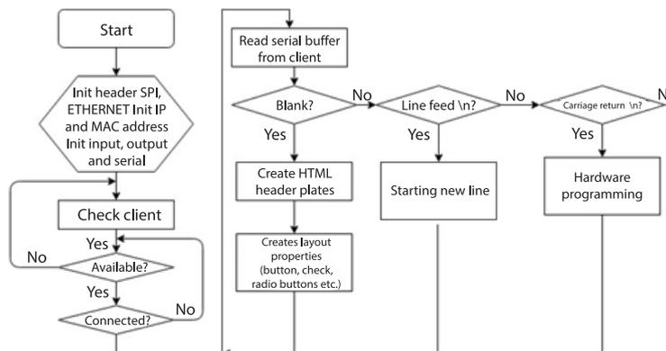
Figure 8. Algorithm flow-chart of solar collector control
