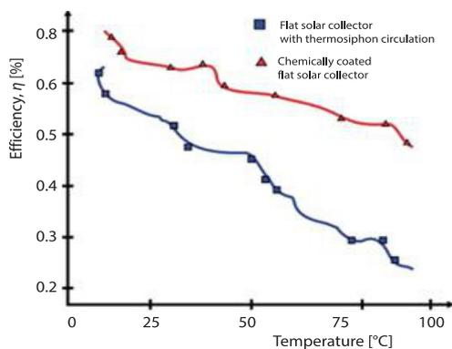
**Figure 9. Efficiency dependence of flat-plate solar collector with thermosiphon circulation and solar collector with chemical coating  $K_2S_2O_8 + NaOH + H_2O + Na_2S_2O_8$**
