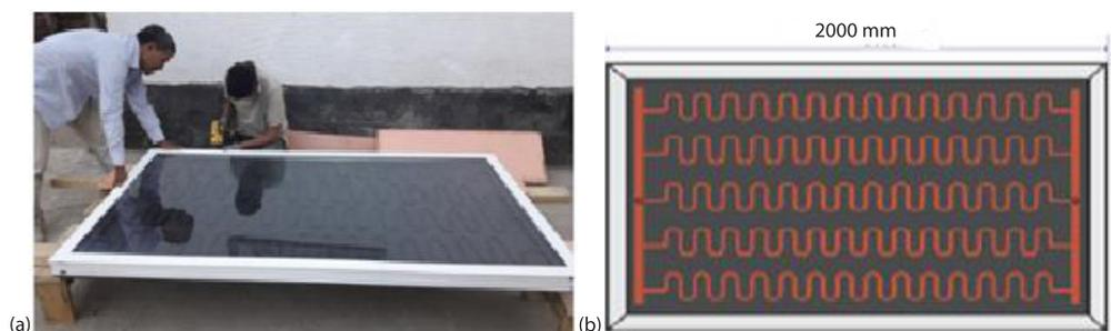
**Figure 3. Solar collector manufacturing processes; (a) flat solar collector with thermosiphon circulation and (b) inner part**
