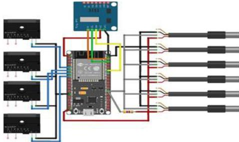
Figure 6. Principal diagram of controller on platform ESP-WROOM-32
