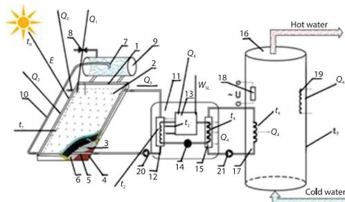
**Figure 1. Principal diagram of double circuit solar installation with thermosiphon circulation**
