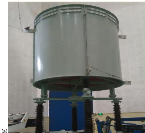
Figure 6. The prototype and temperature rise test results of reactor; (a) prototype of reactor and (b) test results
