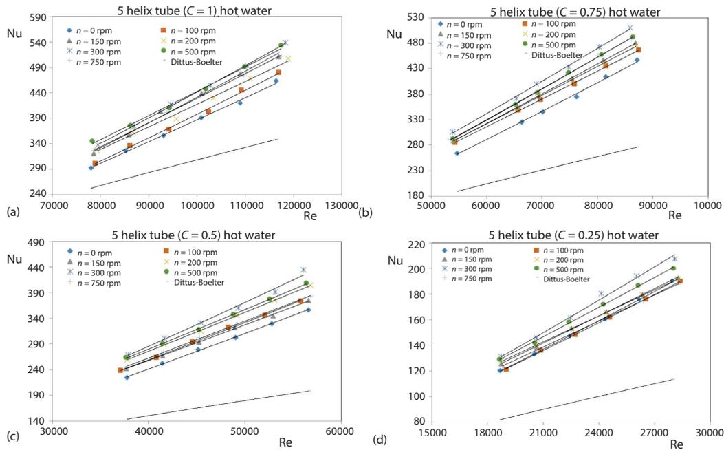
Figure 8. The Nu-Re change for C in 5 helixes tube for hot water; (a) C = 1, (b) C = 0.75, (c) C = 0.5, and (d) C = 0.25
