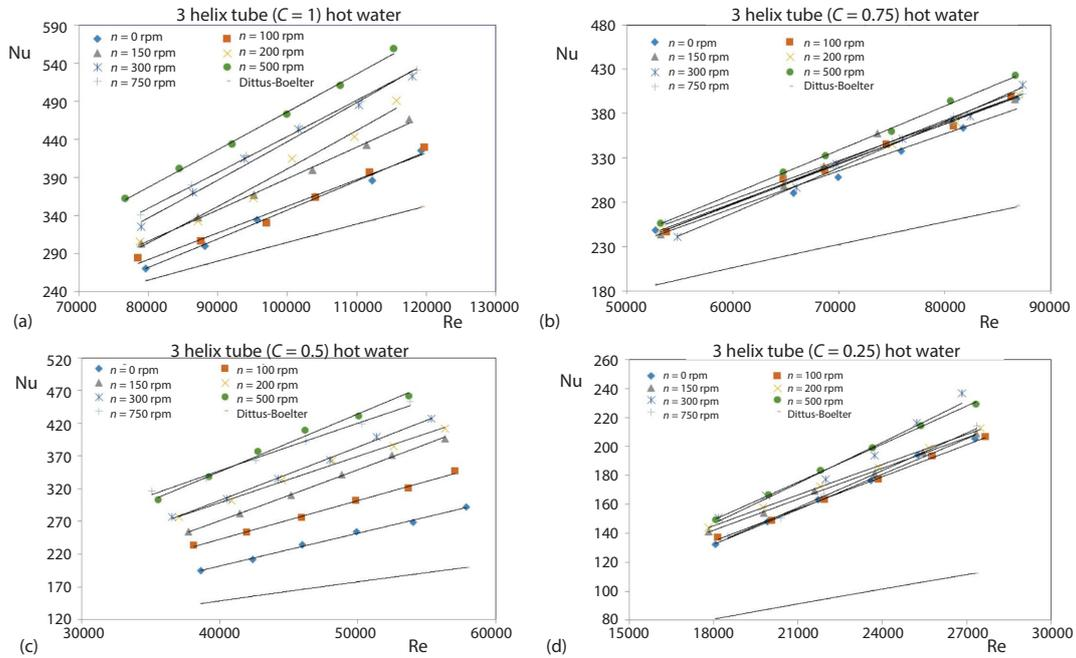
Figure 6. The Nu-Re change for C in 3 helixes tube for hot water; (a) C = 1, (b) C = 0.75, (c) C = 0.5, and (d) C = 0.25
