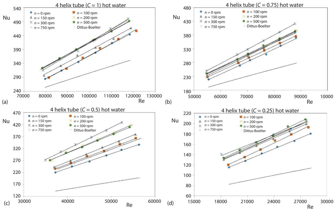
Figure 7. The Nu-Re change for C in 4 helixes tube for hot water; (a) C = 1, (b) C = 0.75, (c) C = 0.5, and (d) C = 0.25
