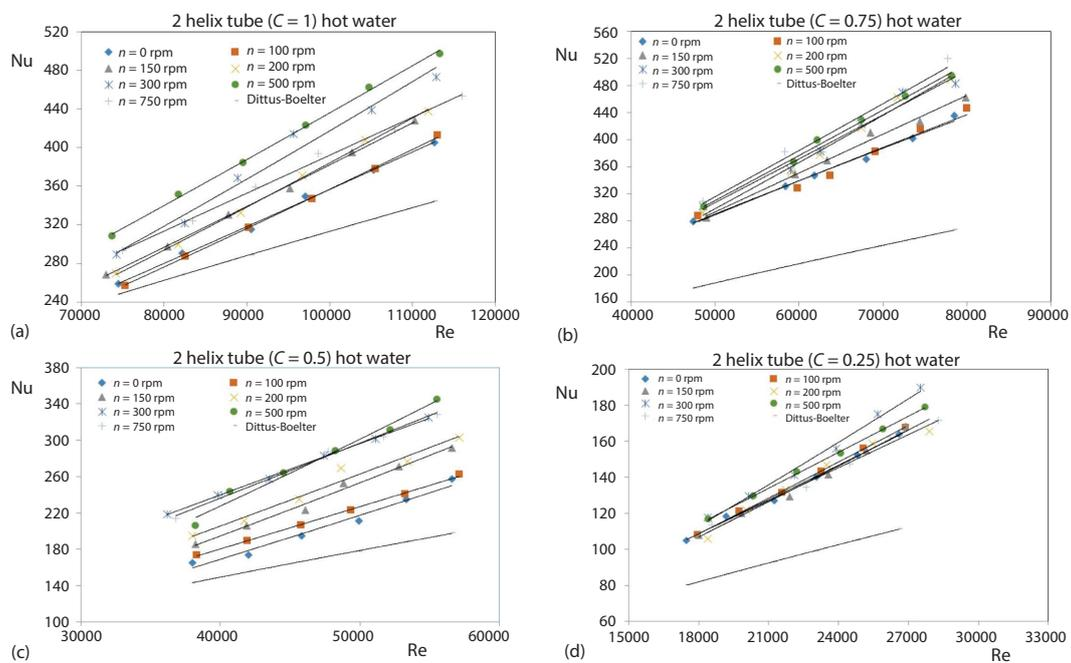
Figure 5. The Nu-Re change for C in 2 helixes tube for hot water; (a) C = 1, (b) C = 0.75, (c) C = 0.5, and (d) C = 0.25
