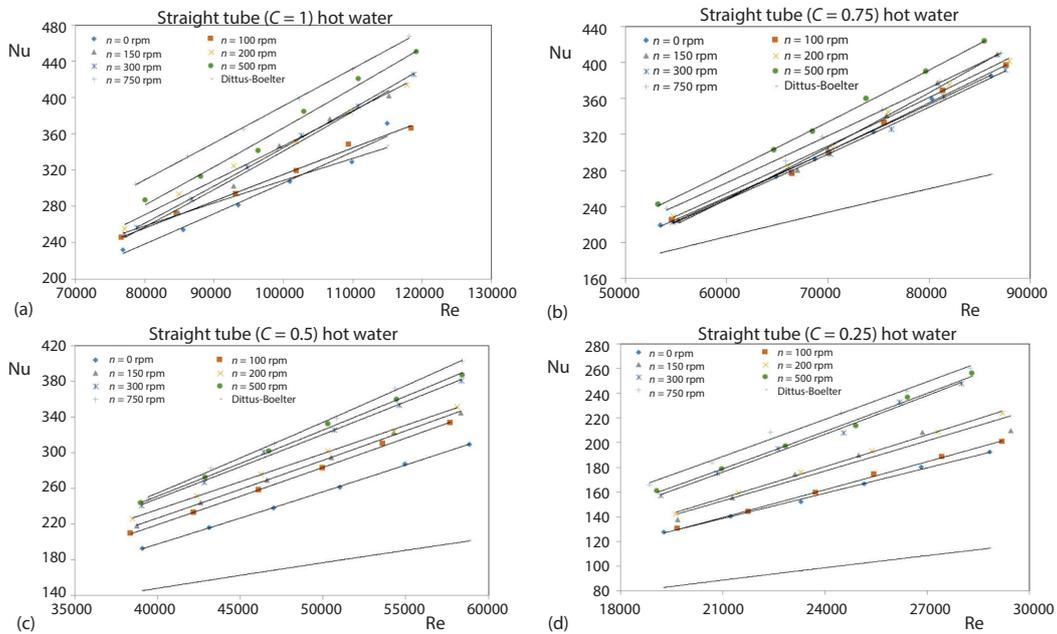
Figure 4. The Nu-Re change for C in straight tube for hot water; (a) C = 1, (b) C = 0.75, (c) C = 0.5, and (d) C = 0.25
