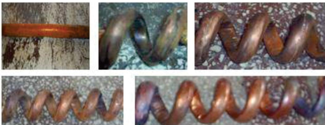
**Figure 3. Different types of inner tubes used in the experiment set**
