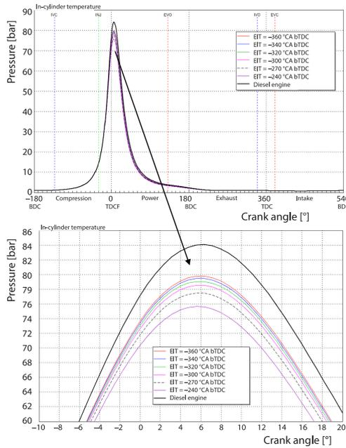
Figure 11. Variation in cylinder pressure with CA at full load according to EIT
