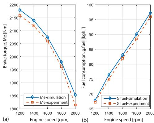
Figure 3. Brake torque and fuel consumption in an hour vs. simulation and experiment at 100% load and engine speeds from 1200-2000 rpm; (a) brake torque and (b) fuel consumption
