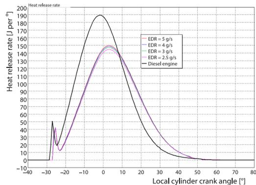
**Figure 14. Variation in heat release rate of dual-fuel engine operation with CA at full load according to the different EDR**
