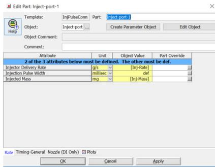
Figure 5. Input interface window of ethanol injector element
