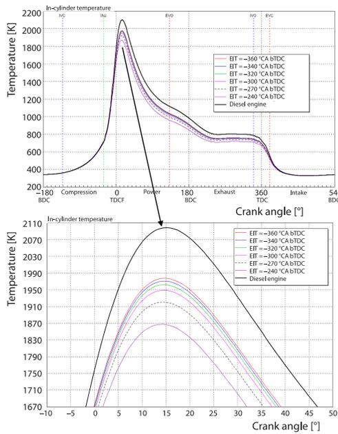
**Figure 9. In-cylinder gas temperature of dual-fuel engine operation with ethanol fumigation according to the different EIT**
