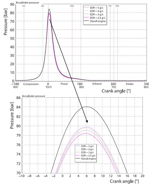
Figure 12. Cylinder pressure of dual-fuel engine operation with ethanol fumigation vs. ethanol injection rates under simulation condition
