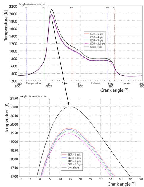
**Figure 10. The in-cylinder gas temperature of dual-fuel engine operation with ethanol fumigation at the different injection rates**
