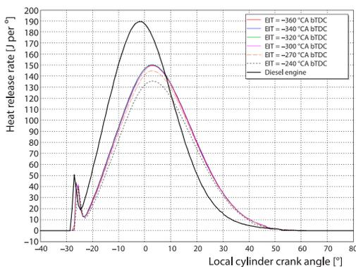
**Figure 13. Variation in heat release rate of dual-fuel engine operation with CA at full load according to the different EIT**
