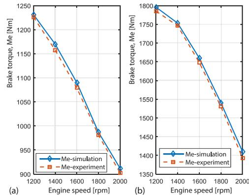
Figure 4. Brake torque vs. simulation and experiment at 50%, 75% load and engine speeds from 1200-2000 rpm; (a) brake torque: 50% load and (b) fuel consumption: 75% load
