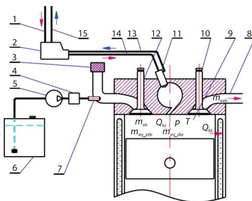
**Figure 1. Schematic diagram of ethanol fumigation system, [11]:**
