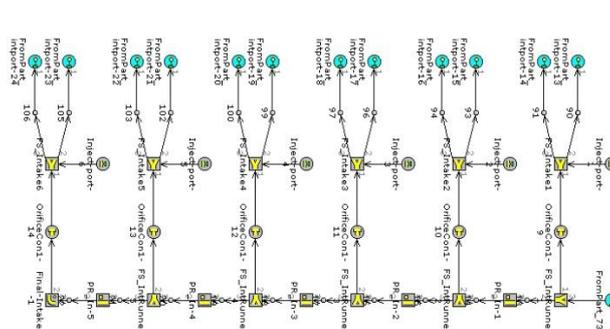
Figure 6. The intake manifold of the dual-fuel engine operation with ethanol fumigation
