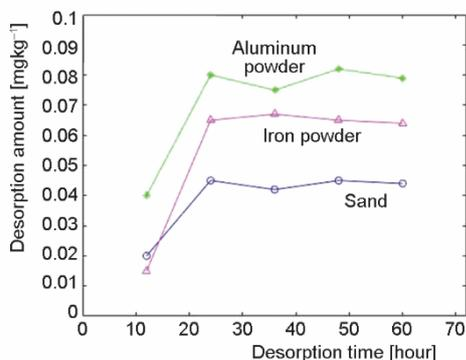
Figure 5. The relationship between the desorption amount of nitrate nitrogen in each media and time
