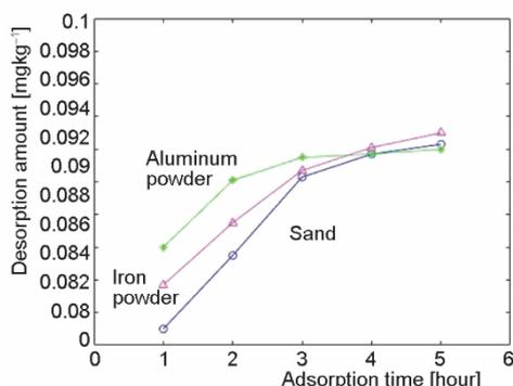
**Figure 6. Kinetic graphs of adsorption of nitrate nitrogen by various media**
