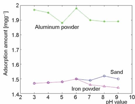
**Figure 3. The adsorption curves of various media at different pH values**
