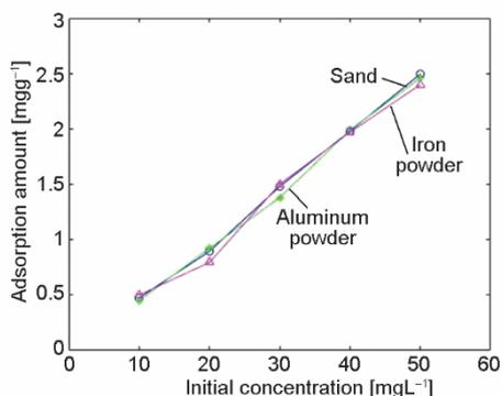
**Figure 1. Isothermal adsorption capacity of different media**
