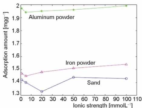
Figure 4. Adsorption curves of various media under different ionic strengths
