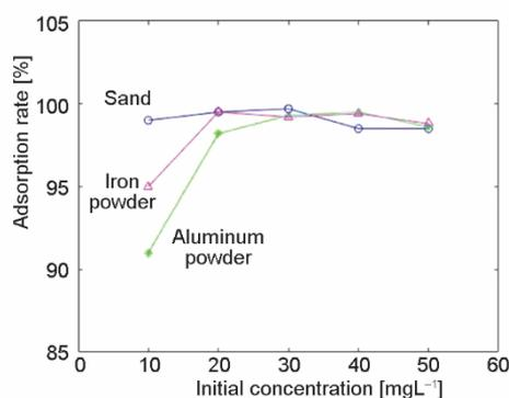
**Figure 2. Isothermal adsorption rate of different media**
